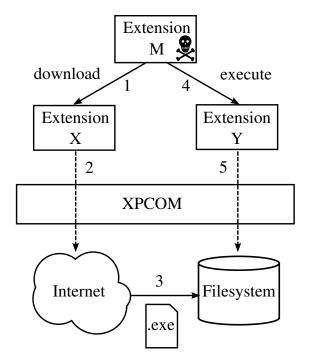
Figure 1. A sample extension-reuse attack showing the malicious extension M reusing functionality from two legitimate extensions to indirectly access the network and filesystem. In this way, the malicious extension discreetly downloads a malicious file and executes it.
